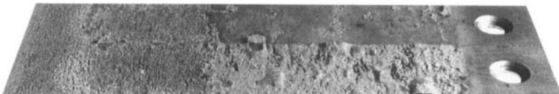
FIGURE 6 Photographs of three fracture surfaces between adherends with a grit-blast plus SCA treatment and tested as follows:
